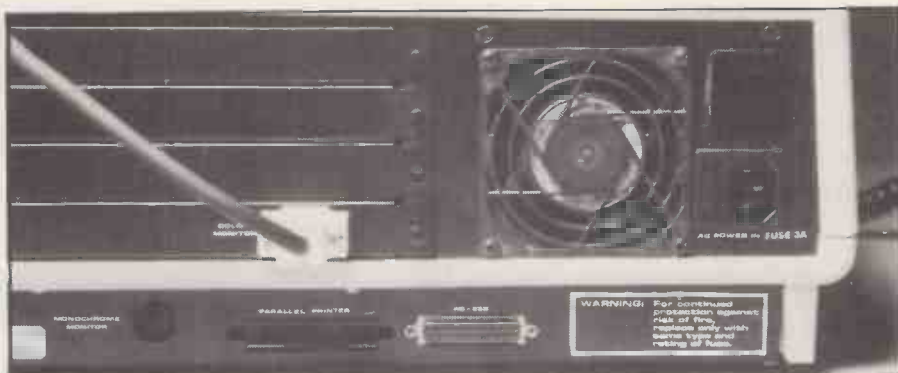
Four removable slots for additional boards lie next to the cooling fan.
